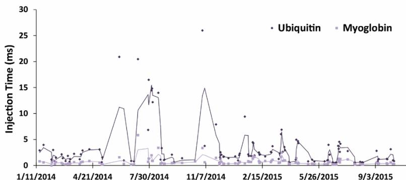
**Example longitudinal data:** Consistent observation of certain metrics, in this case the MS1 injection time (ms) of ubiquitin and myoglobin in TD standards run on the LTQ-Velos Orbitrap Elite, can indicate the onset of ion optics charging or other instrument issues that might otherwise be more difficult to detect.
