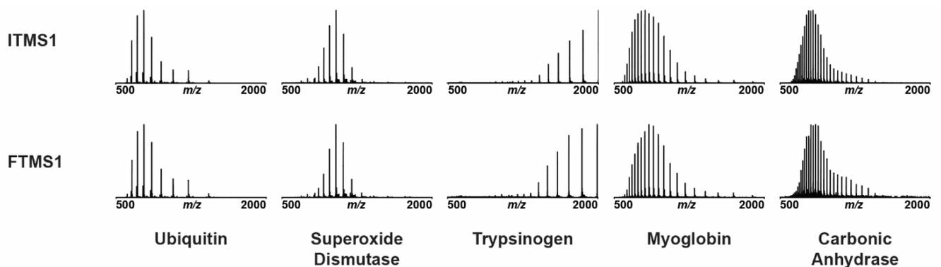
**Example IT and FT MS1 spectra:** Averaged ITMS1 and FTMS1 spectra for each of the five peaks in the above chromatogram (LTQ-Velos Orbitrap Elite), showing the characteristic isotopic peak distributions for each protein. Note the fidelity of the FTMS1 spectra to those acquired in the ion trap; this serves as an indicator of optimal ion transmission and FT performance.
