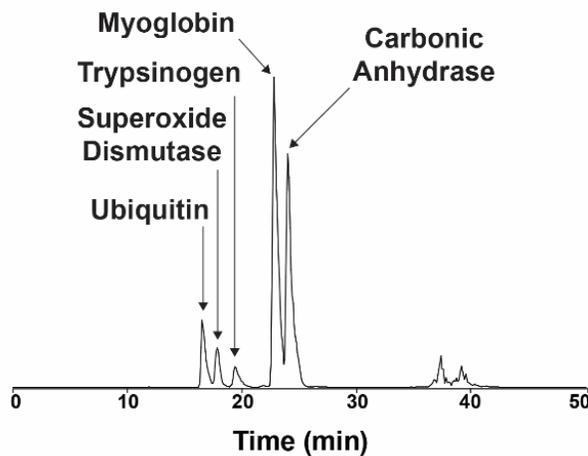
**Example Chromatogram:** Typical base peak chromatogram of the NRTDP TD standard, showing five separate eluted protein peaks (the fifth being due to superoxide dismutase, a characteristic contaminant of carbonic anhydrase). The elution order and relative height ratio of each protein peak should remain consistent. The example shown was obtained on the LTQ-Velos Orbitrap Elite, using the LC and MS parameters described above.
